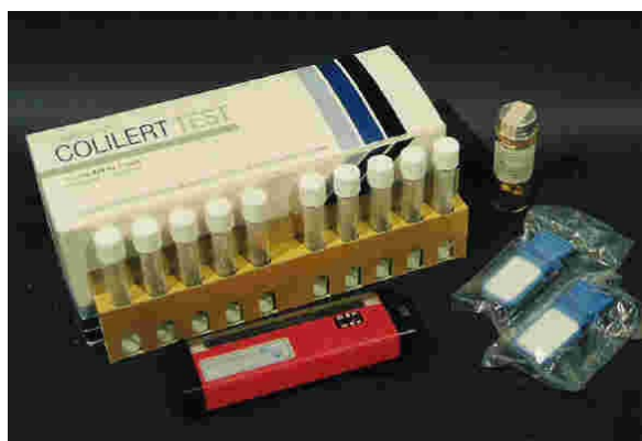
(l-r) Colilert test tubes and fluorescent light; H 2 S strips; Dipslides
